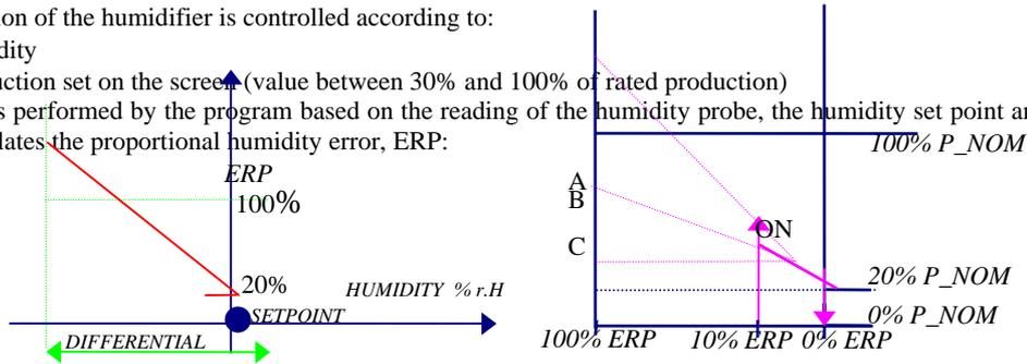
The graph of humidifier production control is based on the rated production, set production and proportional error (ERP):
