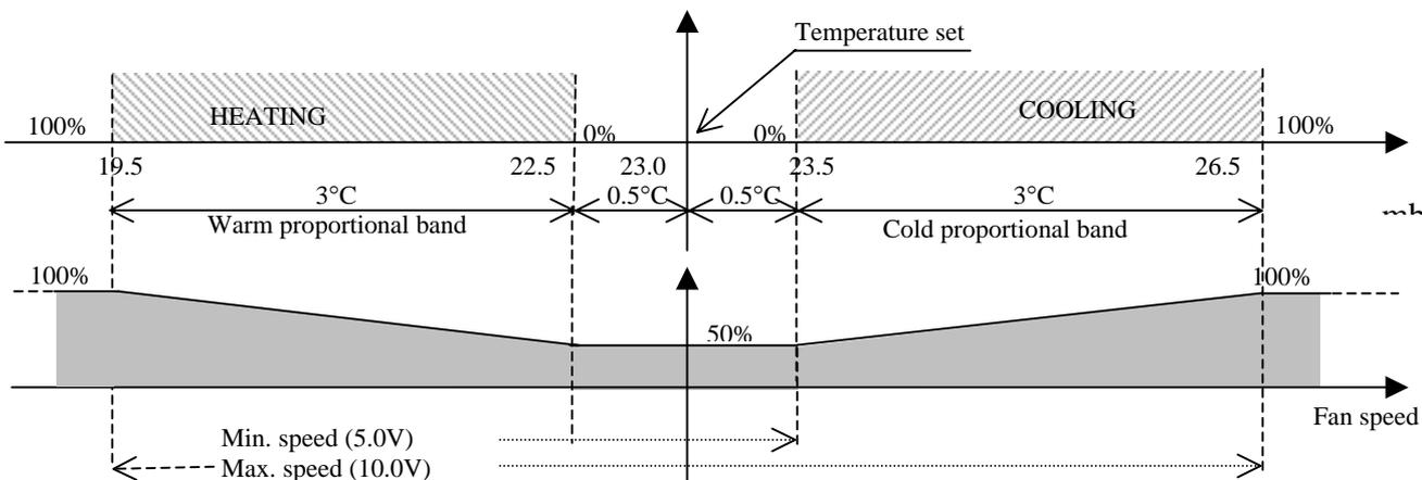
During dehumidification, speed is automatically decreased to 5.0V (50%) default value, modifiable if required. The minimum and maximum speeds default values correspond to 5.0V and 10.0V, modifiable if required.
