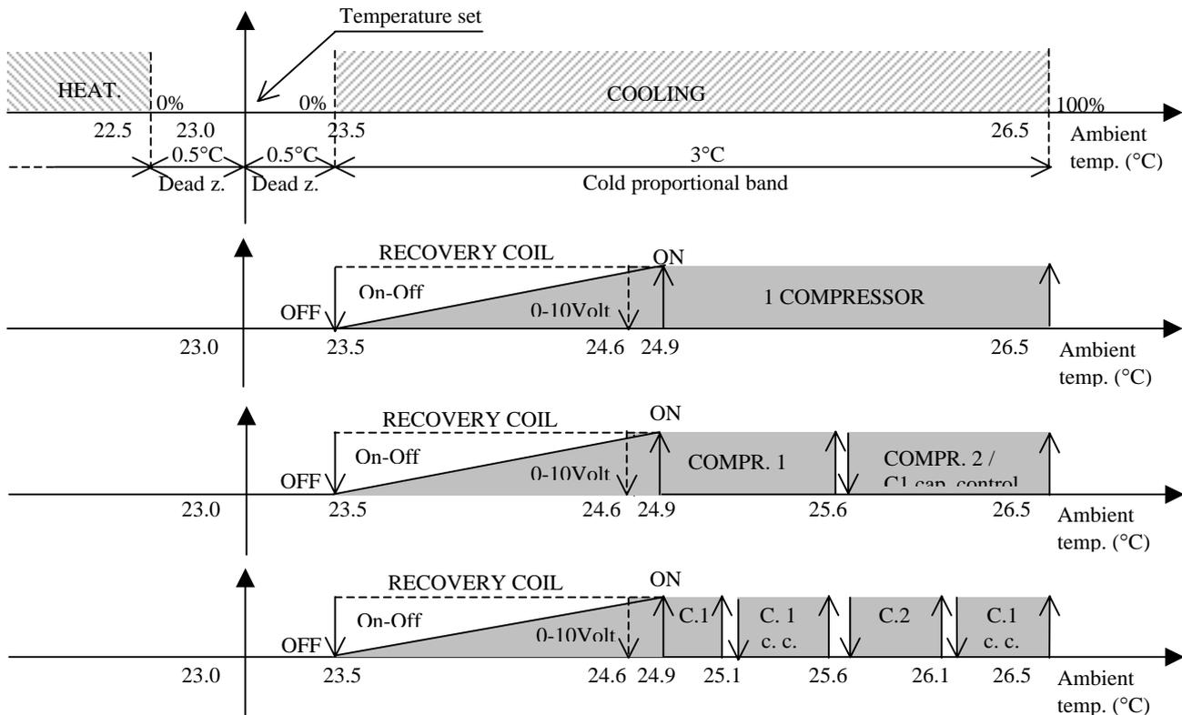
**11.3 RECOVERY WITH COOLING DEVICES ON CLOSE CONTROL UNITS WITH WATER COILS**
