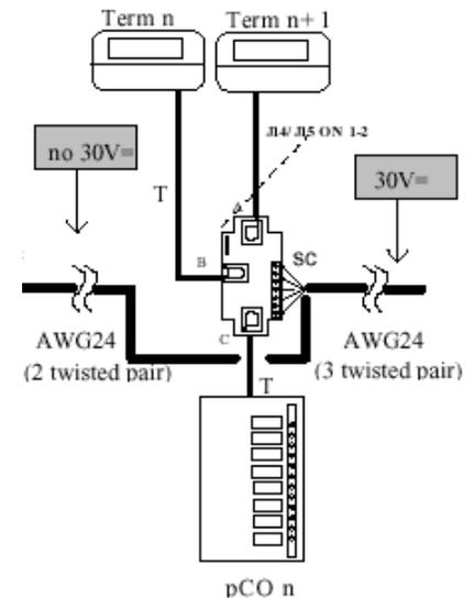
The shared terminal only allows printing all boards alarms and parameters.
