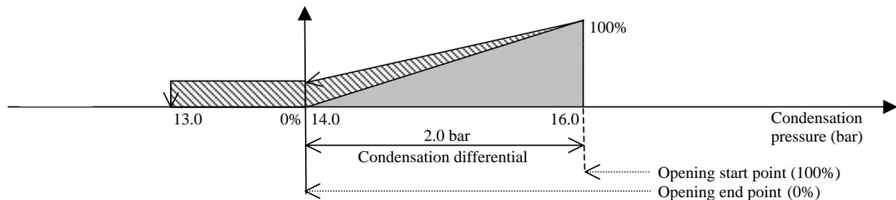
The maximum and minimum speeds of 0-10V outputs can be set; in case the set minimum speed is higher than 0V, the fan is operated at minimum speed 1.0 bar below the condensation set point before switching off, as indicated in the diagram above.
