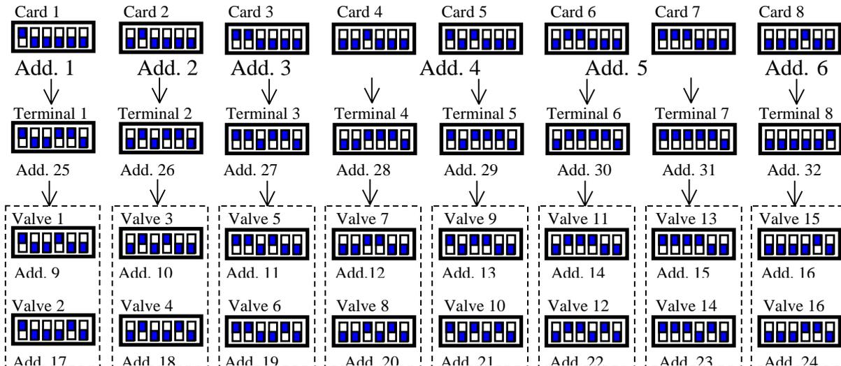
Each external terminal refers to one board and two electronic valves, that is:
