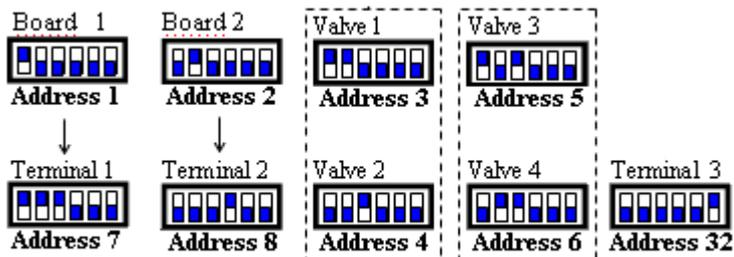
The main Menu screen indicated on the terminals shows the address of the connected card in the bottom left-hand corner. With the ind.32 terminal, all the cards can be controlled without any need for other terminals or in addition to them. In fact, the program enables ind.32 (address 32) terminal to access the parameters of all the connected cards, one at a time. To change over from one card to another, just press the info key.,
