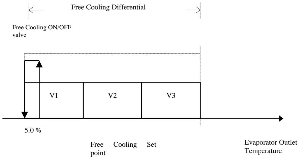
Here is an example of Free Cooling control with ON/OFF valve and three condensation steps.
