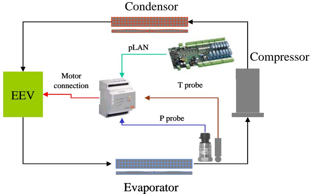
The basic principle of the new control algorithm is to reach the superheating set-point quickly.
