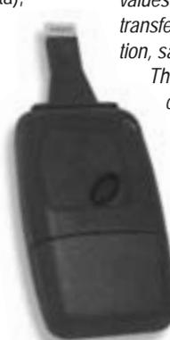
Fig. 9.1.1 During the first 12 seconds the consumption of current is reduced, in that the instrument's LEDs and display are not turned on due to their high consumption.
