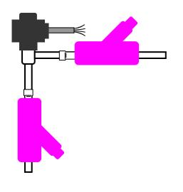
It is strongly recommended the use of a removable filter in the liquid line before EEV refrigerant inlet especially in Supermarket application
