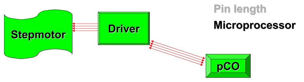
EEV algorithm is on the Driver but in with pCO Sistema it is possibile to customize the EEV action
