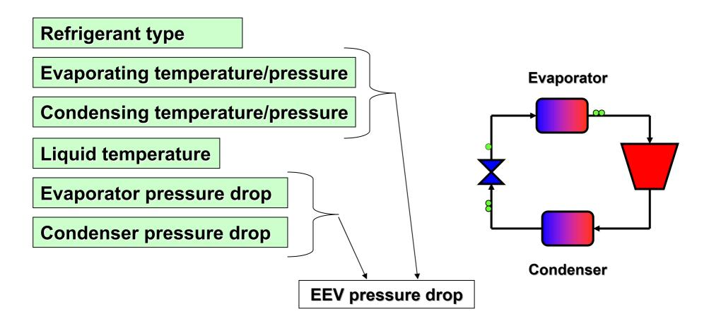
What is necessary to properly size an E<sup>2</sup>V electronic expansion valve?
