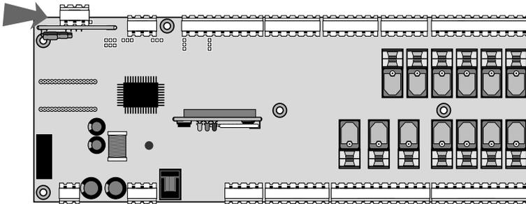
The connection to the RS485 occurs via the card's plug-in connectors.
